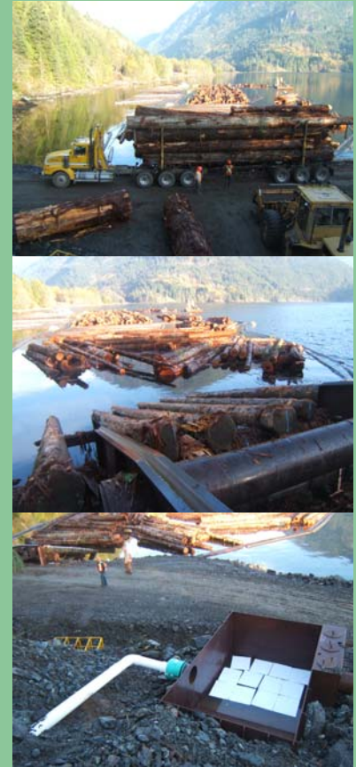
Log dumps visited during the field audit were well designed to minimize environmental risks (e.g., longer, gentler sloped skidways to minimize bark introduction to water during dumping and well located, effectively functioning oil-water separators).
